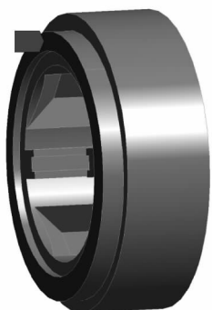
图5 活动套筒与轴承接触面 Figure 5 Contact surface between movable sleeve and bearing
