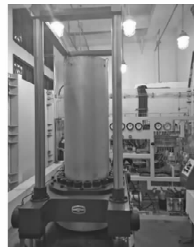
图 1 高压氢环境材料耐久性试验装置 Figure 1 Durability test device for high pressure hydrogen environmental materials
