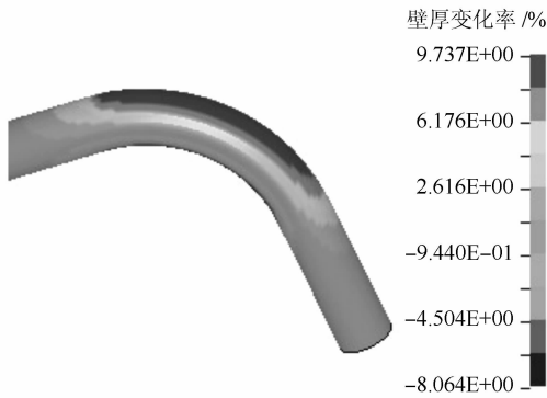
图5 超弹体连接模型壁厚变化率云图 Figure 5 Change rate of wall thickness of super-elastic connecting
