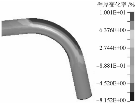
图3 刚体球铰接模型壁厚变化率云图 Figure 3 Change rate of wall thickness of rigid ball hinge
